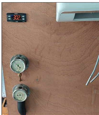
Figure 6. Temperature sensor calibration check in ambient air
