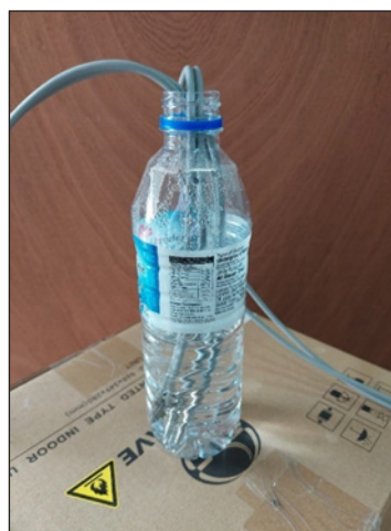
Figure 7. Temperature sensor calibration check in water medium
