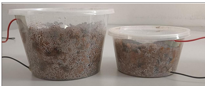
Figure 2. 700 ml and 350 ml MFC chambers
